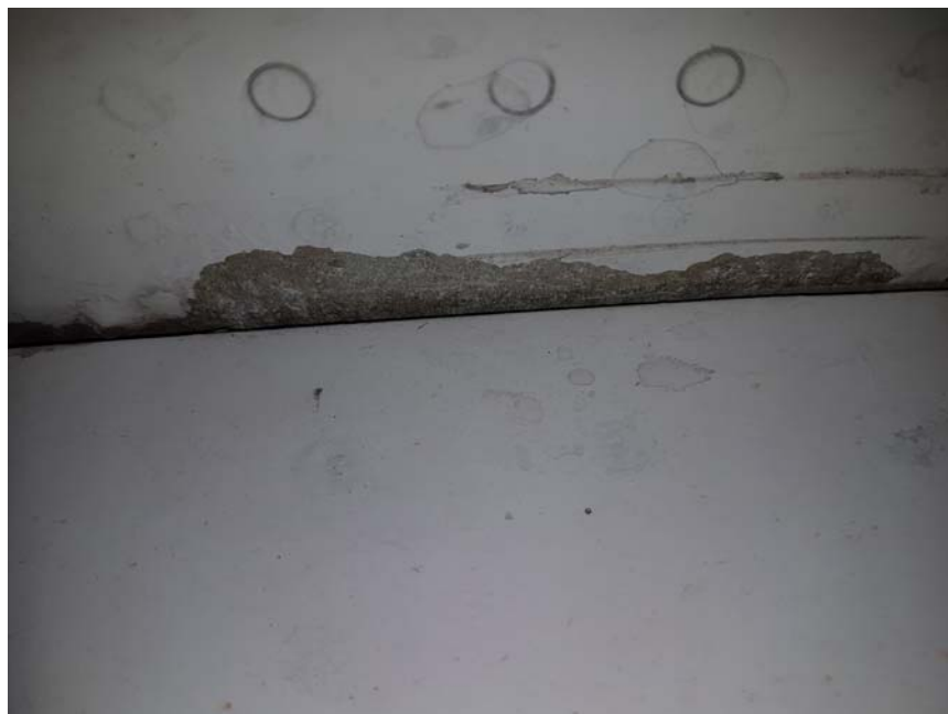
Figure 7. Example of Damage - Wing Skin at Landing Gear Door
