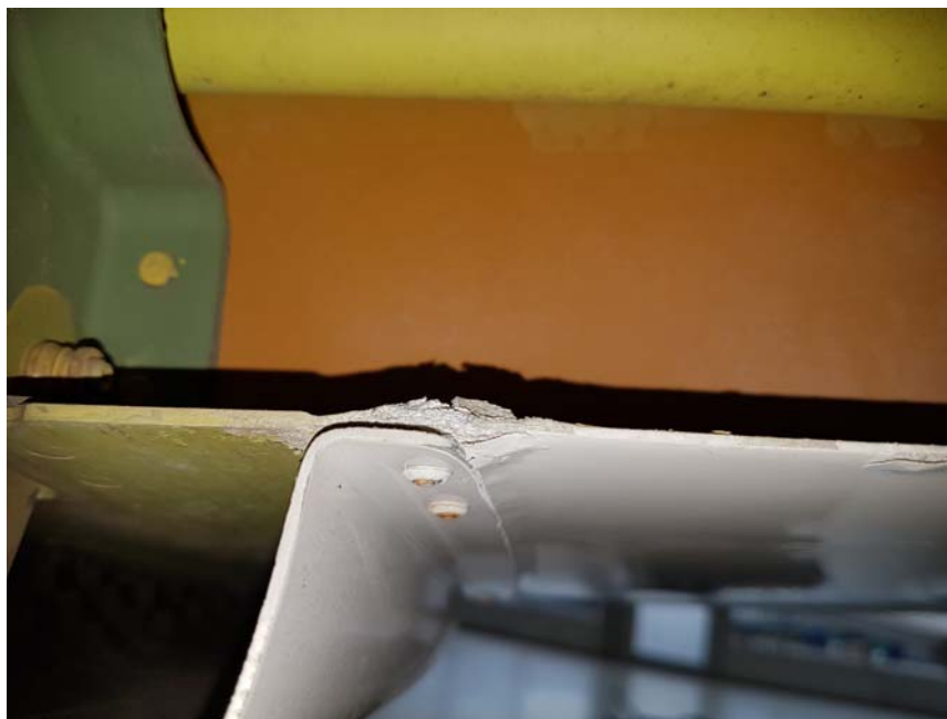
Figure 4. Example of Damage - Outboard Forward Flap Track Fairing
